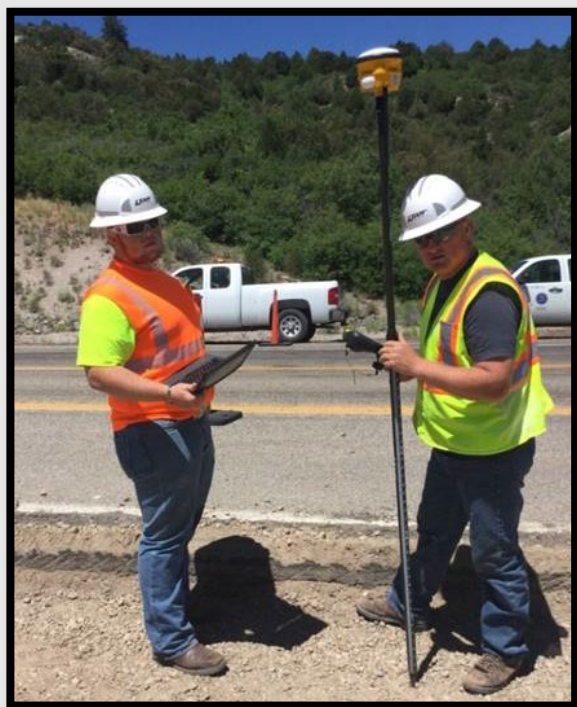
Inspectors use a rover and a tablet to collect survey data electronically.
